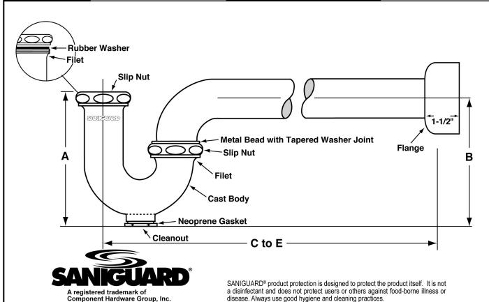
FED SPEC W.W.P. 541 CAST BRASS P-TRAP MINIMUM SEAL 2"
