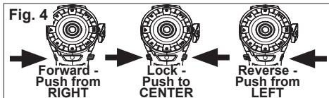
For **forward** (clockwise) rotation, push in the control switch from the right side of the tool. **Check the direction of rotation before use.**
