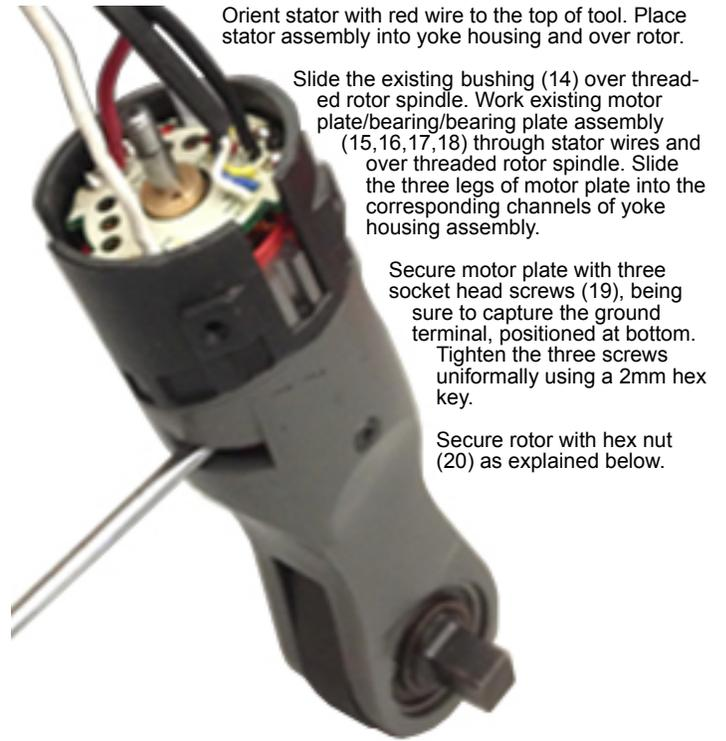
Orient stator with red wire to the top of tool. Place stator assembly into yoke housing and over rotor.
