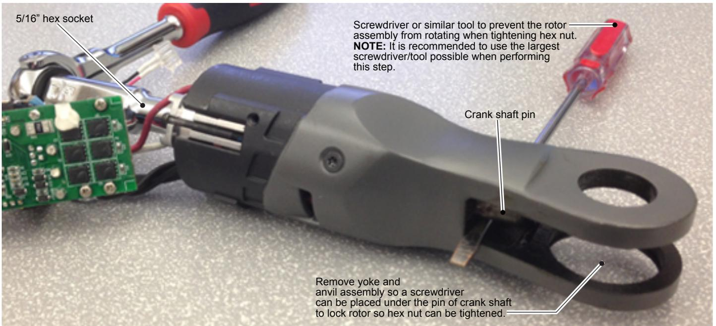
Screwdriver or similar tool to prevent the rotor assembly from rotating when tightening hex nut. **NOTE:** It is recommended to use the largest screwdriver/tool possible when performing this step.
