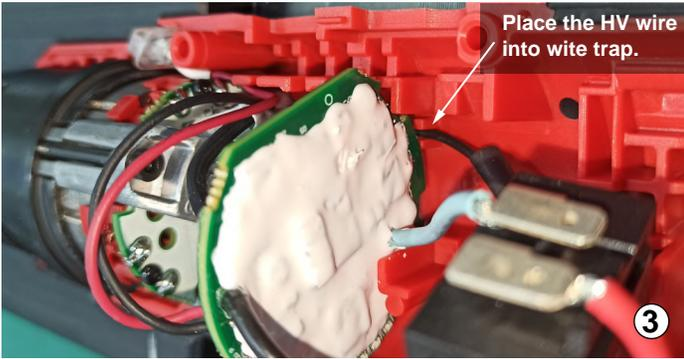
Assemble control board into housing slot.
