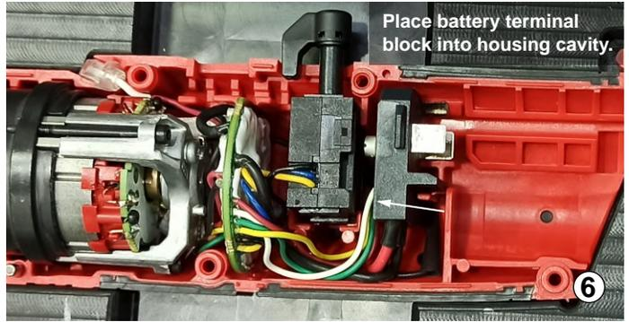
Push all wires down into housing cavities as shown.
