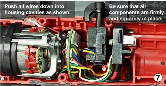
Install the switch lock-out slide
