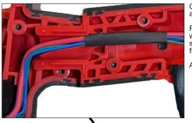
Carefully place/route ribbon cable in traps as shown
