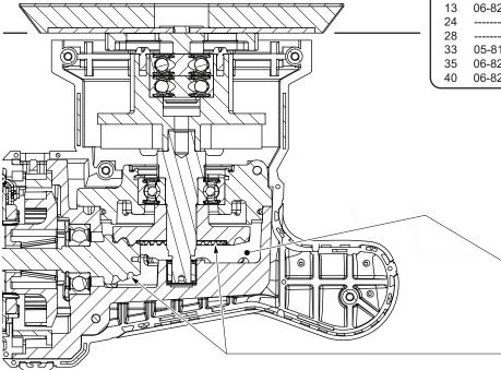
**SCREW TORQUE SPECIFICATIONS SEAT TORQUE** FIG. PART NO. WHERE USED (KG/CM) (IN/LBS) 5 06-82-2380 Gear Case 22±2.0 19±2.0 10 05-88-1300 Gear Case 20±2.0 17±2.0 06-82-0135 Shroud Cover 10.0±1.0 8.5±1.0 Lower Counterweight 15±1.5 13±1.5 17±2.0 Upper Counterweight 20±2.0 05-81-1160 Reciever Plate 10±1.0 8.5±1.0 06-82-0251 **Backing Plate** 25±2.5 21.5±2.5 06-82-1076 Foot Support 14±1.5 12±1.5
