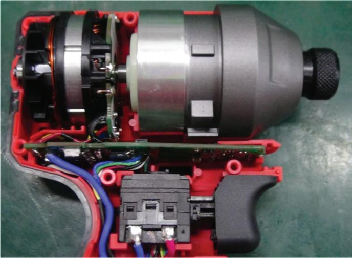
**STEP 7:** Assemble gear box/impact assembly onto rotor pinion. Be sure gear box, rotor and stator are firmly and squarely seated in left housing half and that the rotor fan has movement.
