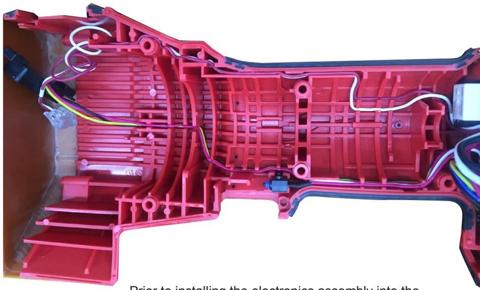
Prior to installing the electronics assembly into the housing support, place grounding terminal over screw boss as shown. Route ground wire, removing as much slack as possible. Be sure wire is pressed firmly to the back of the wire traps.
