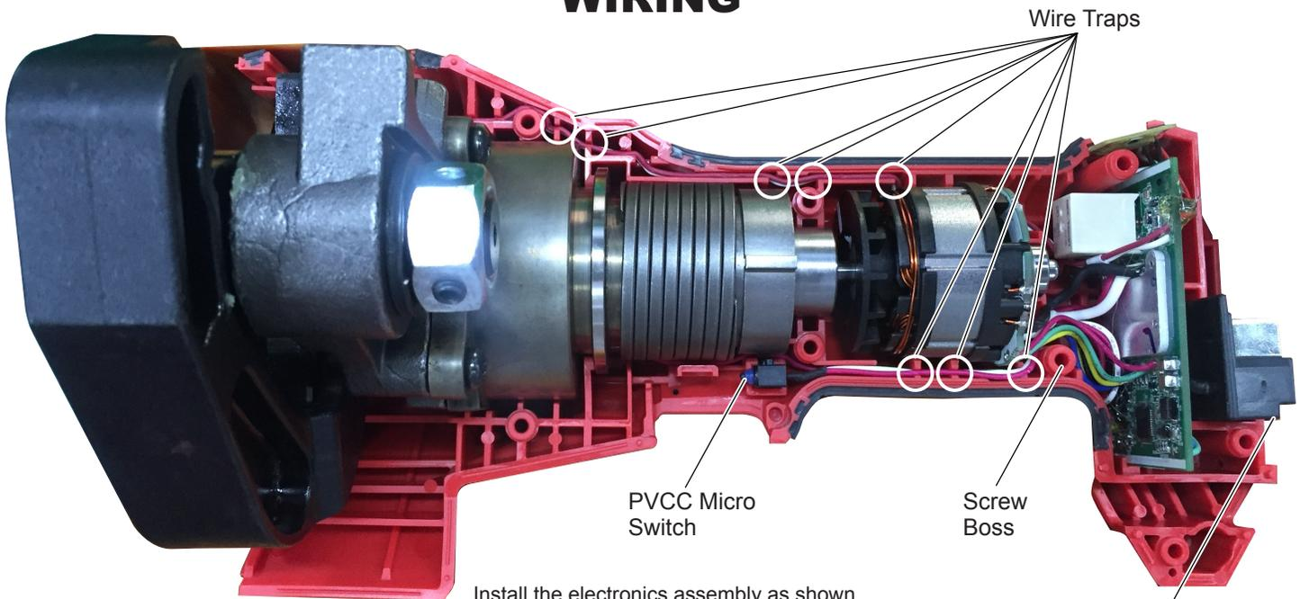
Install the electronics assembly as shown. Route wires around screw bosses and into wire traps. Be sure all components are seated squarely and firmly in place. Be sure there is no interference when installing the housing cover.
