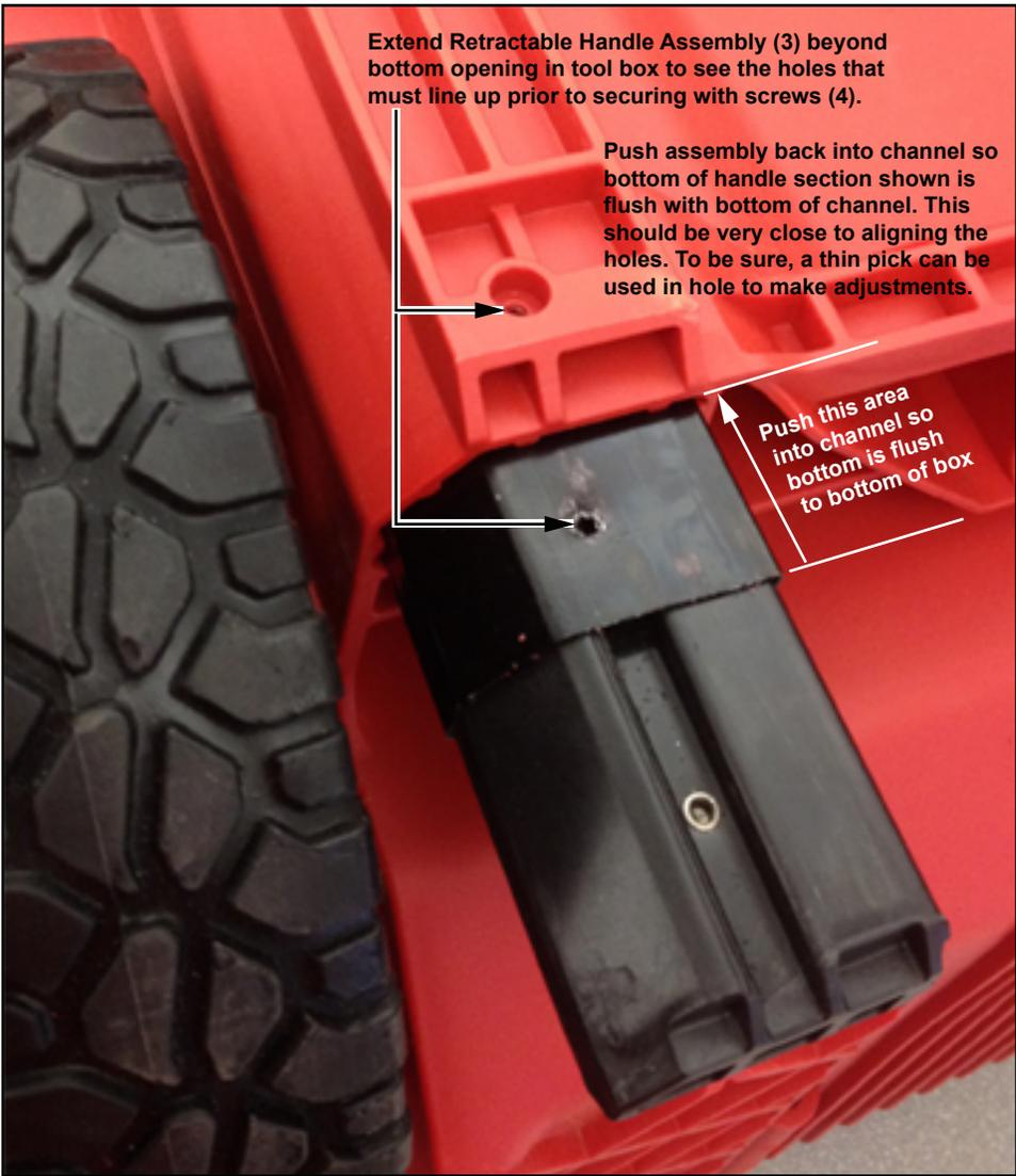
Extend Retractable Handle Assembly (3) beyond bottom opening in tool box to see the holes that must line up prior to securing with screws (4).
