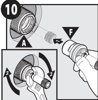
1. Insert Replacement Cartridge (F) into Flow Valve (A).
