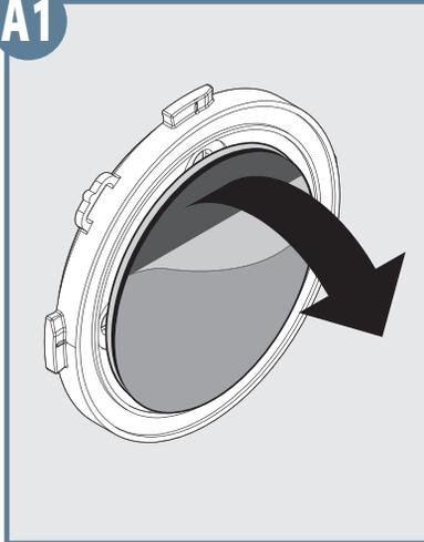
Peel away the adhesive liner from the back of the magnetic dock's wall bracket. Stick it to the wall, and firmly push it in place for about 1 minute. For optimal adhesive strength, allow to cure 24 hours before sliding the dock onto the bracket.
