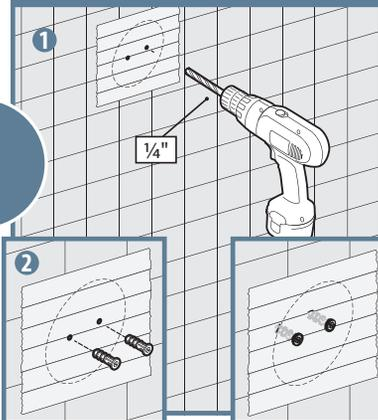
**For Tile:** Use a 1/4" drill bit, not included, and drill holes on the marks. Insert the anchors into the holes.
