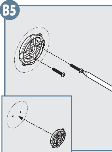
Place the bracket on the wall and fasten using the screws.
