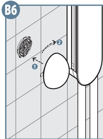
1. Take the dock with tab on top and install over the bracket.
