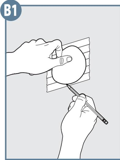
Using a pencil, lightly trace a circle around the dock onto the wall or painter's tape.
