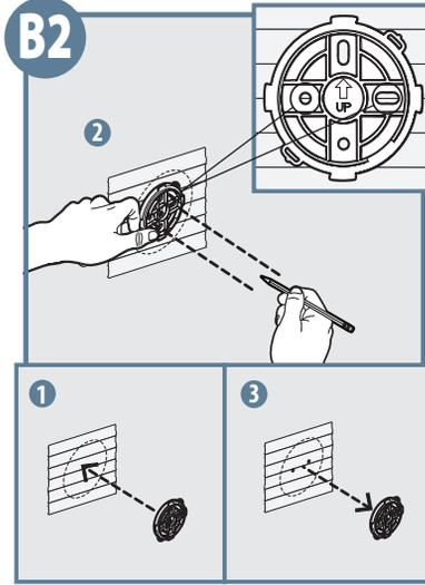
Center the bracket within the marking. Mark the center of the left and right holes. Remove the bracket from the wall.
