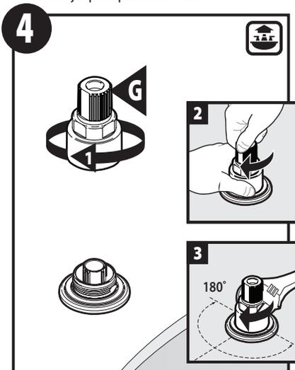
1. Thread Handle Adapter (G) onto handle rough-in, flat side of splines to face away from spout.
