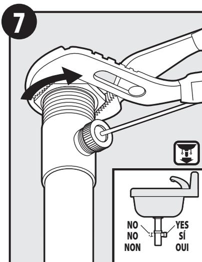
Make final tightening of drain nut with channel locks or an adjustable wrench. Ensure drain body opening faces back of sink as shown in inset illustration.
