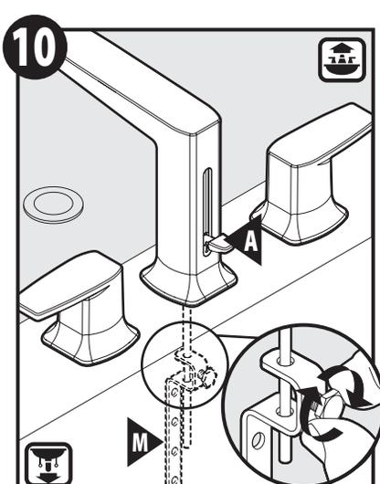
Insert Lift Rod (A) into Lift Rod Strap (M). Tighten Lift Rod Strap (M) by hand.
