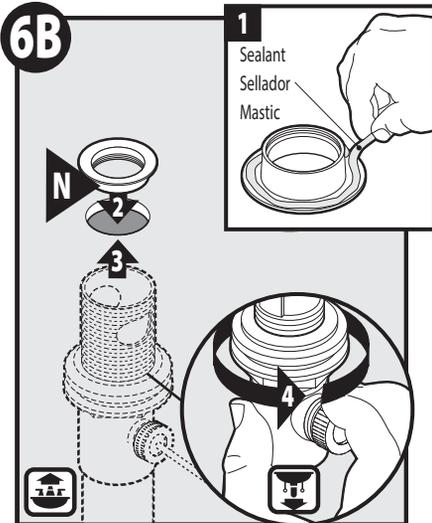
1. Apply sealant to underside of Waste Seat (N).
