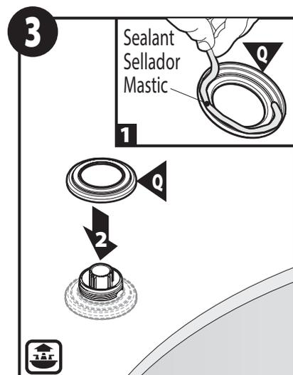
1. Apply sealant to underside of Handle Escutcheon (Q).
