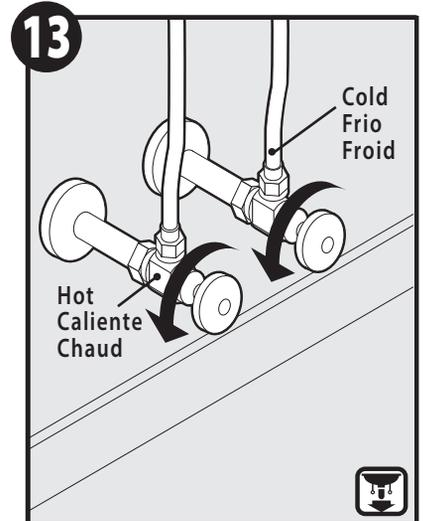
Turn on water, check for leaks.
