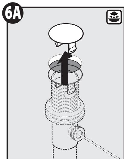
To complete waste connection, remove drain snap-in holder.
