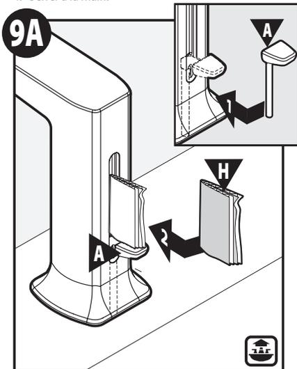
1. Insert Upper Lift Rod (A) thru spout slot.
