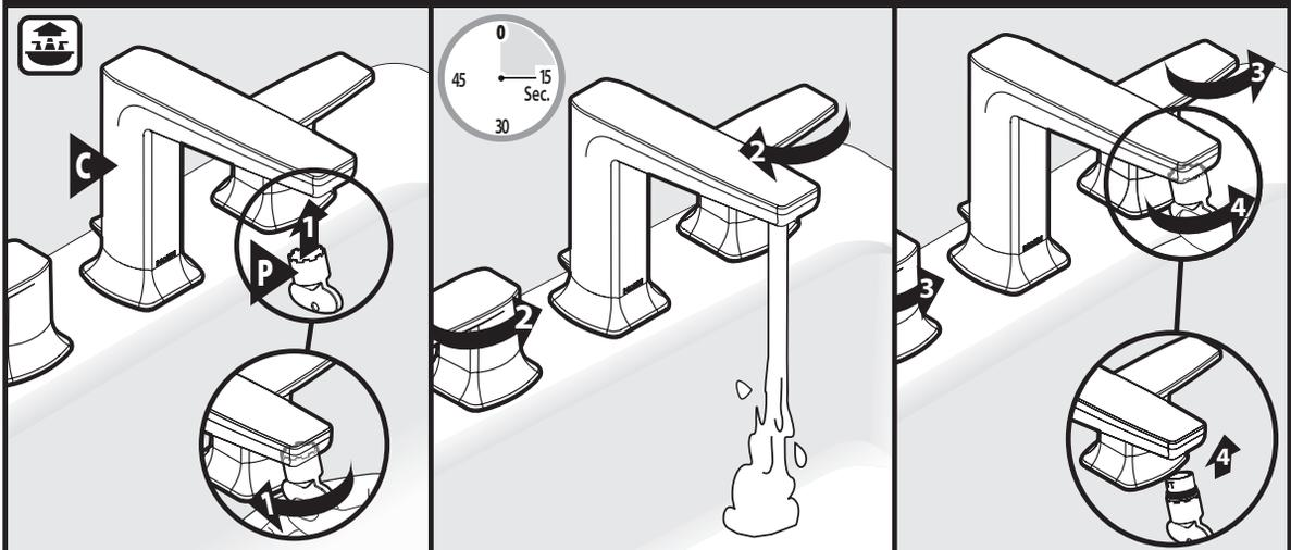
1. To flush debris from the plumbing system: Remove the aerator by using the included aerator tool (P).
