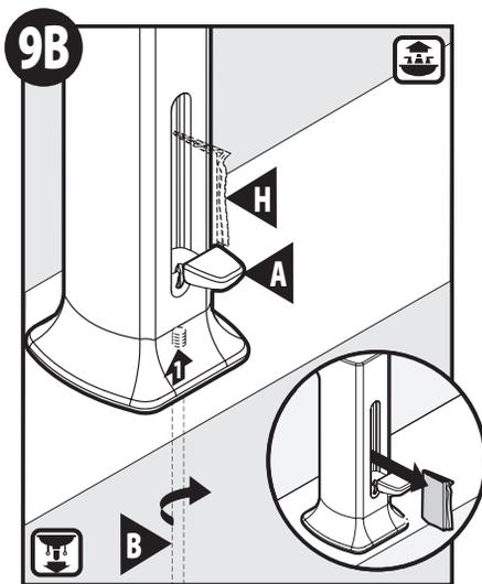
1. From under deck, thread Lower Lift Rod (B) into Upper Lift Rod (A).
