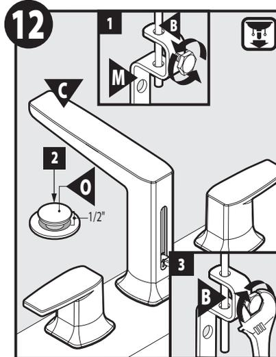
1. Loosen bolt on Lift Rod Strap (M).
