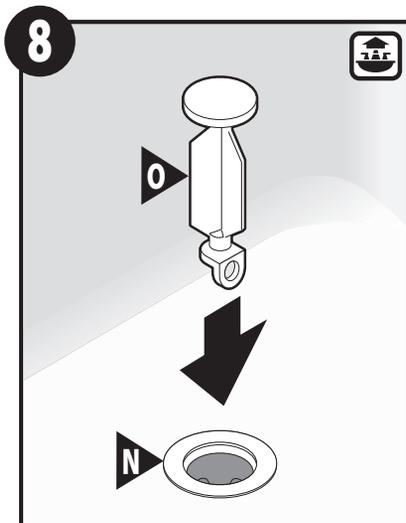
Insert Drain Plug (O) into Drain Waste Seat (N).
