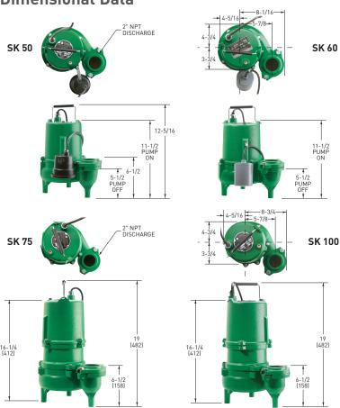
All dimensions in inches. Metric for international use. Component dimensions may vary ± 1/8 inch. Dimensional data not for construction purpose unless certified. Dimensions and weights are approximate. On/Off level adjustable.
