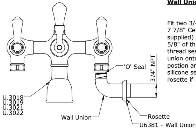
Fit two 3/4" NPT female fittings into the wall at 7 7/8" Centers. Fit a 3/4" NPT male shank (not supplied) into the fitting so that no more than 5/8" of thread is protruding from the wall. Apply thread sealing material to shank and screw union onto shank. Turn union to required position and slide rosette up to wall surface. A silicone seal can be applied between the wall rosette if required.
