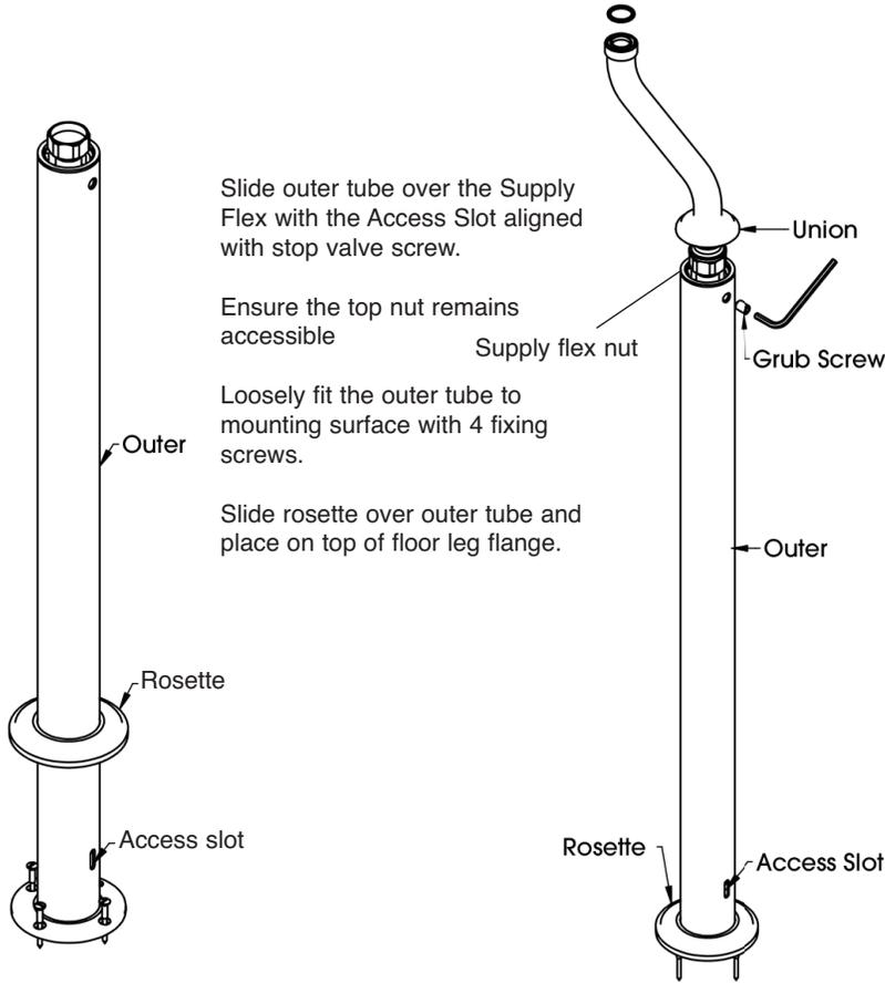
Slide outer tube over the Supply Flex with the Access Slot aligned with stop valve screw.
