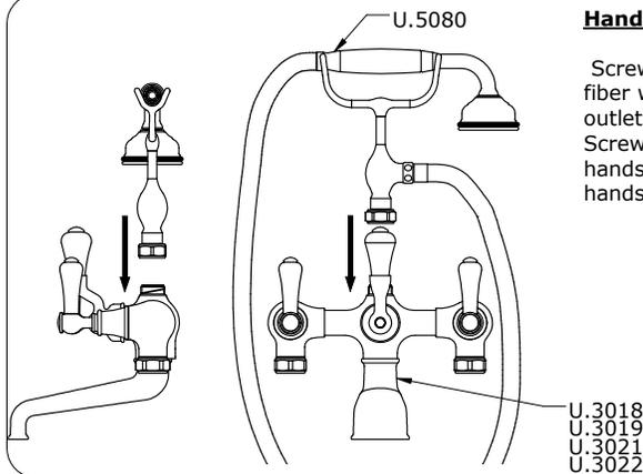
Screw cradle nut fully onto the mixer body, ensuring that the fiber washer is in position between the cradle and body. The outlet for the handshower can be positioned facing left or right. Screw tapered end of the handshower hose onto the handshower and screw the nut end onto the cradle. Place the handshower onto the cradle.
