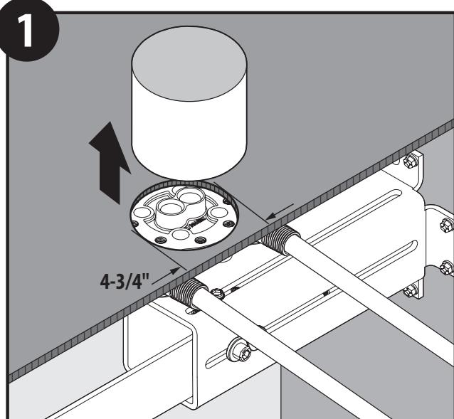
Remove mud cover from manifold assembly to install tub filler.
