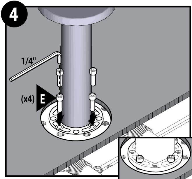
Tighten 4 Screws with Washers (**E**) with 1/4" hex key.
