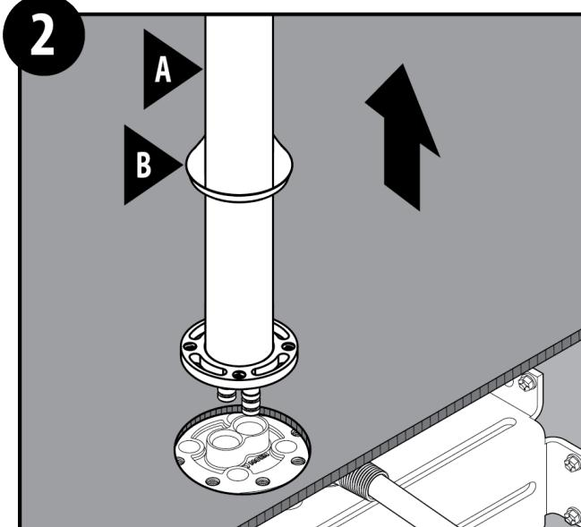
Slide Riser Escutcheon (B) up the Tub Filler (A).
