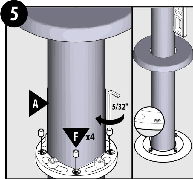
Level Tub Filler (**A**) using 4 Leveling Screws (**F**).
