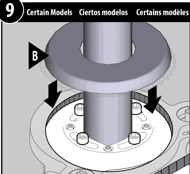
Apply sealant to underside of Riser Escutcheon **(B)**. (Note: On models without floor seal, sealant will be used on the riser escutcheon). Slide the Tub Filler **(A)** to the floor. Ensure the 4 screws are snug to engage the seal. (Note: On some models, ensure to remove protective riser bag).
