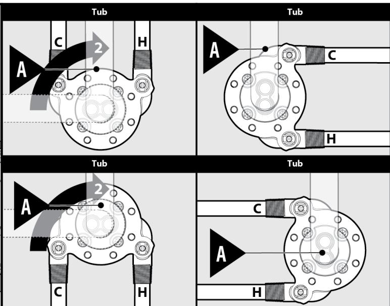
Install Tub Filler (A) to manifold. If pipes are perpendicular to tub: rotate Tub Filler (A) up to 90° so that it faces the tub.
