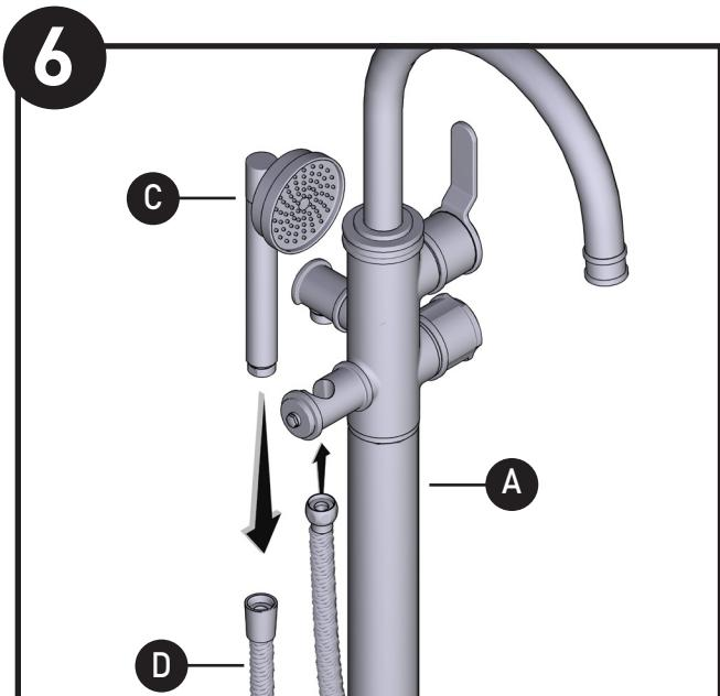
Install the Handshower (**C**) onto the Hose (**D**). Install the other end of the Hose onto the Tub Filler (**A**). Style varies by model.
