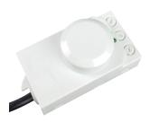
The High Frequency Motion Sensor uses high frequency waves to detect motion. The sensor sends out waves that bounce off nearby surfaces and return to the sensor. Motion changes the speed of the waves returning to the sensor. The sensor detects the change in speed and interprets it as occupancy which causes the light to turn on. It triggers primarily through movement of people, objects, machinery. The band of frequency that it usually operates in is <10 mW (about 10x lower than
