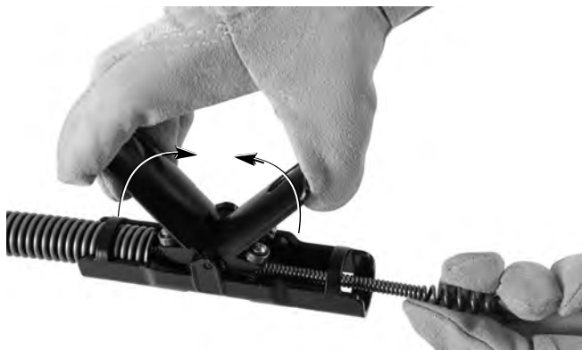
Figure 5 – Feeding Cable Through AUTOFEED® Assembly
