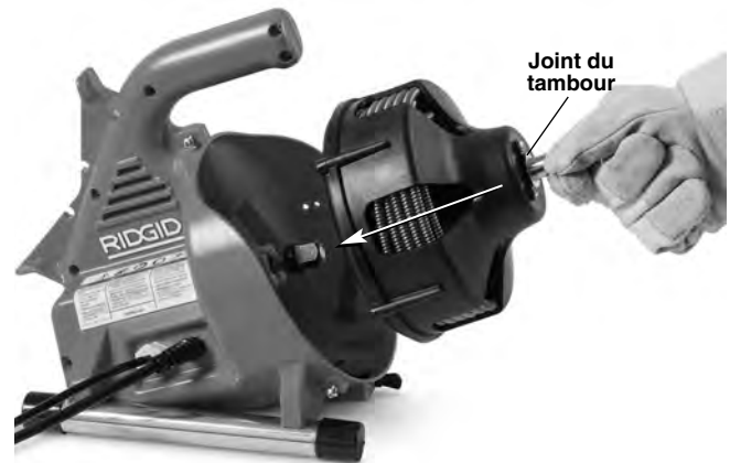
Figure 16 – Insertion du joint de tambour
