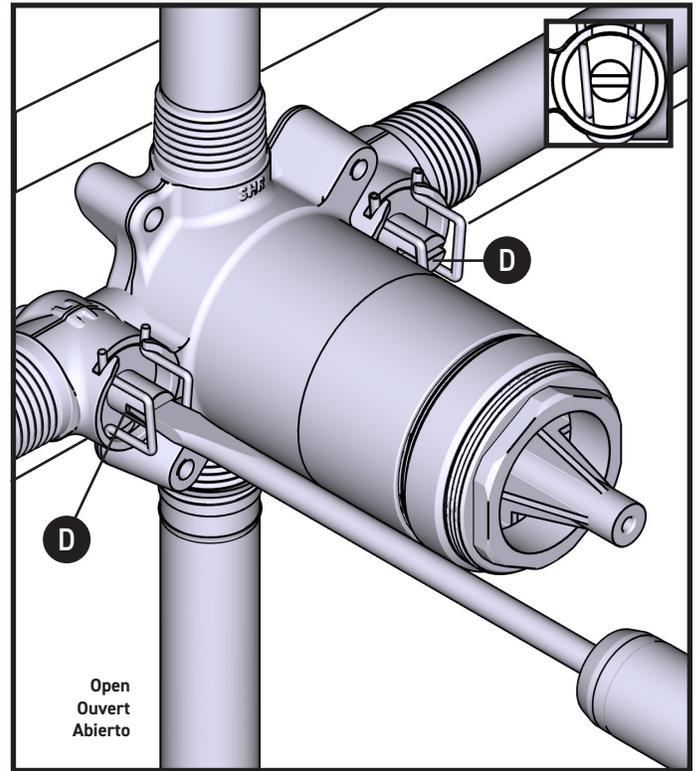
1. Using a flathead screwdriver, rotate the Service Valves (D) to the open position. (Illustration shown is the closed position.)
