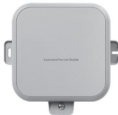
ERM5220R Equipment Remote Module provides wireless RedLINK communication between condensing unit/compressor or boiler and thermostat. Use it whenever it's too costly or time-consuming to run wires from a condensing unit or boiler to control devices. Suitable for outdoor use. Temperature sensor terminals for outdoor temp sensors or indoor freeze protection. LEDs for easy installation checkout.
