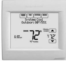
**VisionPRO® 8000 with RedLINK® technology is a touchscreen thermostat, 7 day programmable and selectable for residential or light commercial use. Controls up to 3-stages of heat and 2-stages of cool in a heat pump system and up to 2-stages of heat and 2-stages of cool in a conventional system.**
