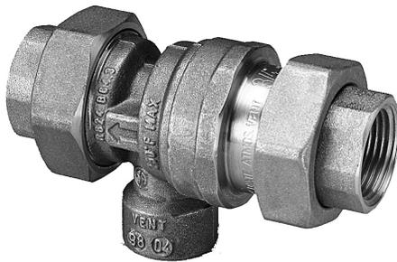
The BP900 backflow preventer is designed for continuous pressure applications on small supply lines. It uses an intermediate vacuum breaker to protect against backflow and back siphonage of contaminated water into potable water supplies.
