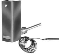
L8100 are immersion type controllers for regulating and limiting the tank temperature in water heater and hydronic systems. As the water temperature rises past the setpoint, the controller switches off the gas valve.
