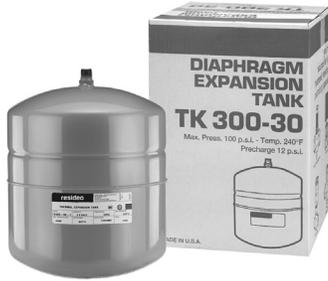
Expansion Tanks absorb hot water expansion in closed heating systems. They are equipped with butyl diaphragms to separate the air from the system water. Pre-pressurized, the tank keeps fluids circulating and maintains minimum pressure.
