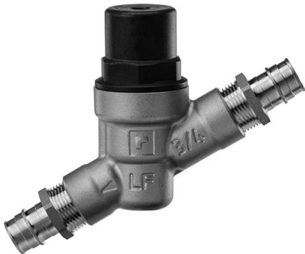
The Resideo Braukmann DS05 is a high-quality balanced pressure regulating valve that maintains a constant outlet pressure over a wide range of inlet supply pressures. It has a simple design with NPT or pre-assembled Push Connect and PEX F-1960 fittings. Available in 3/4-in. and 1-in., the six SKUs require no additional parts, making it a low-cost go-to for every new construction. It is suitable for potable water and irrigation applications, both indoor and outdoor.
