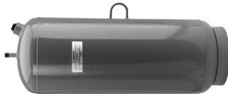
**TAX Series (commercial) Expansion Tanks** are designed to absorb hot water expansion in closed heating systems of large installations. TAX tanks are equipped with butyl diaphragms to separate the air from the system water (glycol).
