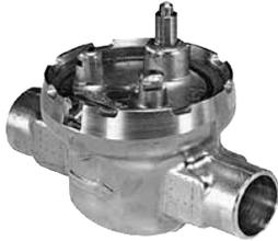
Two-way fan coil zone valves are used to control hot or chilled water in commercial HVAC equipment such as fan coil units, terminal reheat coils and convectors. Not for use in systems containing dissolved oxygen.
