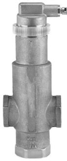
The SuperVent, purges air through a no clog vent assembly, to control dirt and debris and minimize air vent fouling in Hydronic heating systems, while eliminating the need for bleeding.
