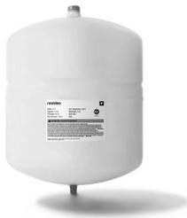
The Thermal Expansion Absorber is an expansion tank with a butyl diaphragm. The Thermal Expansion Tank controls pressure build-up in the system, eliminates relief valve spillage, protects fixtures and extends water heater life.
