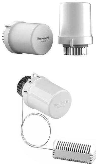
Thermostatic radiator heads are self-actuating controllers which regulate the flow of hot water through thermostatic radiator valves to continuously control the room temperature to the set-point selected on the head.
