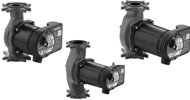
The PC3F in-line, wet rotor circulator with universal flange is designed for applications in closed-loop hydronic heating and cooling systems, as well as in solar systems. The pump is non-submersible and for use in dry, frost-free, well-ventilated installations.
