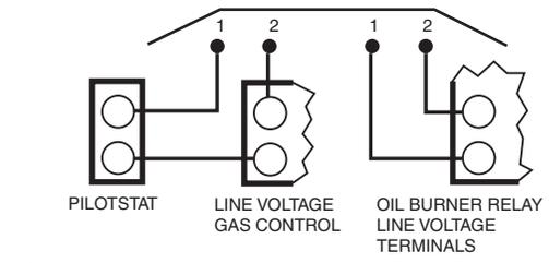
⚠ POWER SUPPLY. PROVIDE DISCONNECT MEANS AND OVERLOAD PROTECTION AS REQUIRED.
