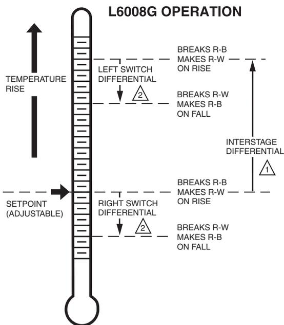
1 DIFFERENCE BETWEEN THE TEMPERATURES AT WHICH THE TWO SWITCHES MAKE R-W. ADJUSTABLE FROM 3°F TO 10°F (1.7°C TO 5.6°C) ON STANDARD MODELS, OR FROM 3.6°F TO 12°F (2.0°C TO 6.7°C); 55°F TO 175°F (13°C TO 79°C) MODELS.
