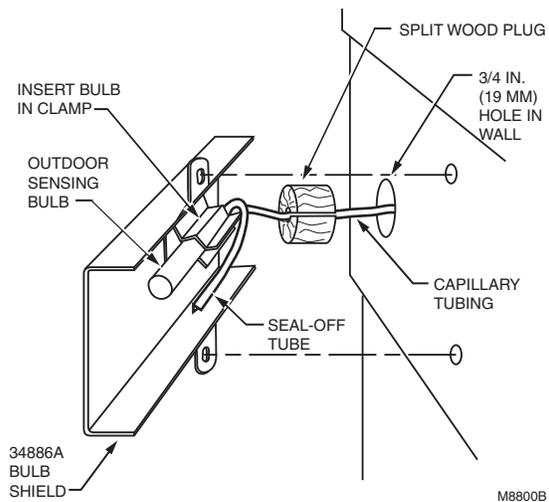
Fig. 15. Mounting bulb in shield outside building.
