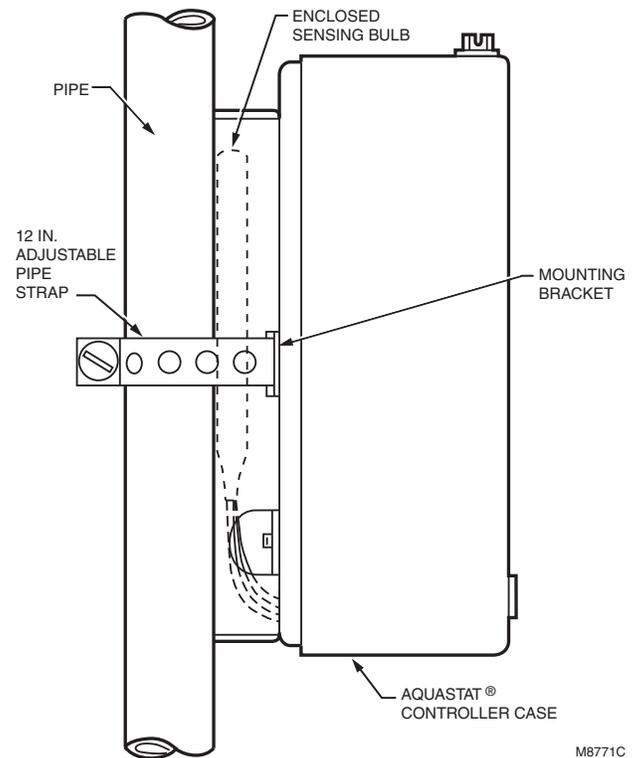
**Fig. 18. Mounting L4006H or L6006C directly on surface.**
