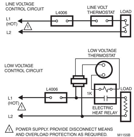
**Fig. 26. Typical systems with 120 volt electric heat primaries.**
