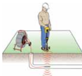
Find sondes (remote transmitters).
