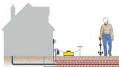
Direct connect to utility lines.
