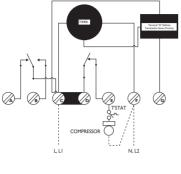
9145 AIR DEFROST - Time Initiated Time Terminated - Wiring Diagram
