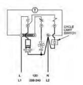
Wiring using 120V or 240V single phase line with compressor thermostat closed during defrost.
