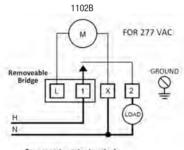
For separate motor terminals remove bridge from terminal L & 1.
