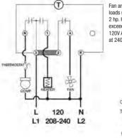
Fan and compressor loads not to exceed 2 hp. Heater not to exceed 4000 watts at 120V AC or 8000 watts at 240V AC
