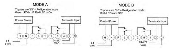
Applying power (24-277V AC) between Terminate Input terminals "X" and "C" causes the unit to return to Refrigeration Mode. If the Terminate input voltage is removed while the trippers are ON, the unit remains in the Refrigeration Mode. The unit remains in Refrigeration until both the Terminate input voltage is removed and the trippers cycle OFF then ON again.
