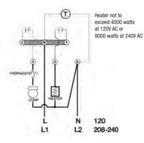
Models 8041-00 and 8041-20 - Wiring Diagram
