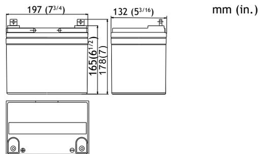
Tolerances are +/-1/32 in. (+/-1mm) and +/-3/32 in. (+/-2mm) for height dimensions.
