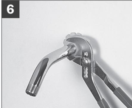
Hold Shower WallNut and thread a **brass shower arm** completely into FIP threads. DO NOT use thread sealant or PT.F.E. tape on Shower WallNut end of shower arm.
