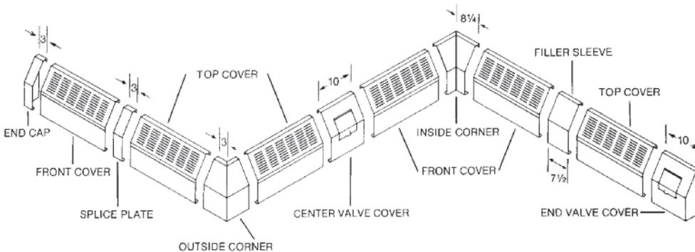
Fourteen accessories let you "fit" Multi/Pak 90 in virtually any space configuration - fast and easily. External cover accessories are all telescopic. They snap in place without screws or other fasteners. All accessories, unless noted, are finished in Nu-White baked enamel. Custom color available on special order.
