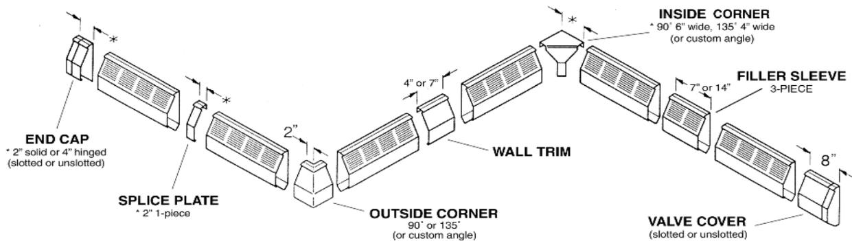
Matching snap-on accessories let you speed through virtually any job condition without custom cutting and fitting. Piano hinged accessories permit easy access with flush or recessed installations.
