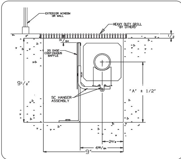
Slant/Fin Trough Heater is a floor recessed commercial finned tube heater. It is ideal for applications with windows coming to the floor, installation by doors or just applications where the building owner does not want visible finned tube. For installations by windows, the cold convective air generated by the window is caught and heated in the natural convective air currents created by the Trough Heater. Cold drafts will be minimized or eliminated. No noise and no electricity.
