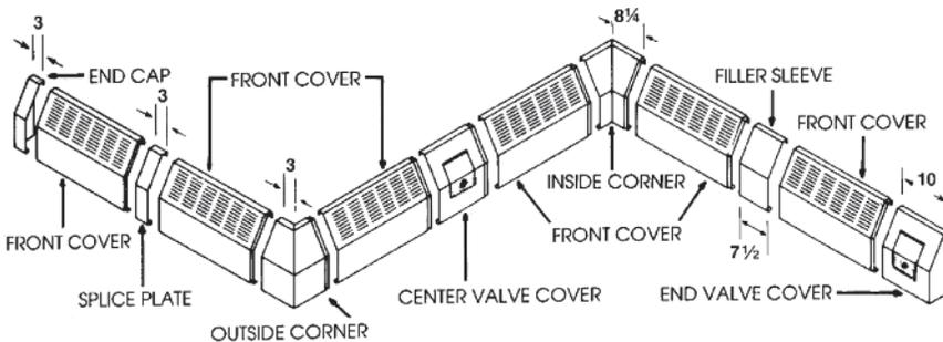
A complete range of accessories lets you "fit" J-series in virtually any space configuration - fast and easily. Cover accessories are all telescopic. They snap in place without screws or other fasteners. All accessories have gray prime finish. Custom color available on special order.
