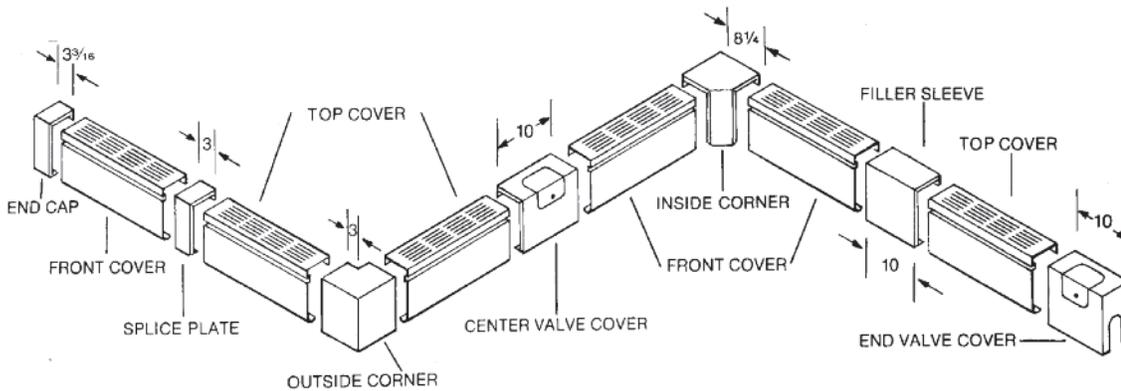
Fourteen accessories let you "fit" Multi/Pak 95 in virtually any space configuration – fast and easily. Cover accessories are all telescopic. They snap in place without screws or other fasteners. All accessories, unless noted, are finished in Nu-White baked enamel. Custom color available on special order.
