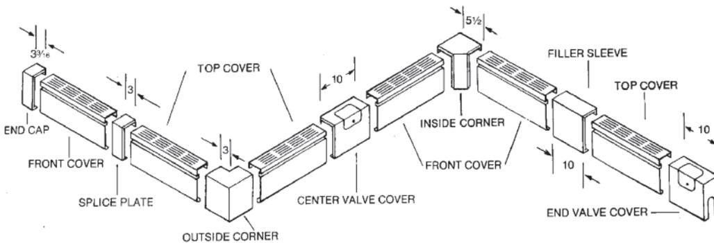
Fourteen accessories let you "fit" Multi/Pak 93 in virtually any space configuration – fast and easily. Cover accessories are all telescopic. They snap in place without screws or other fasteners. All accessories, unless noted, are finished in Nu-White baked enamel. Custom color available on special order.
