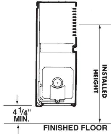
The **installed height** for enclosures is defined as the distance from the finished floor to the center of the outlet. Recommended height is based on a minimum mounting height for all covers and enclosures of 4¼" from finished floor to bottom of front panel.
