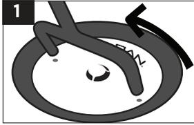
1 Insert Key into cartridge, turn key to left to unlock.
