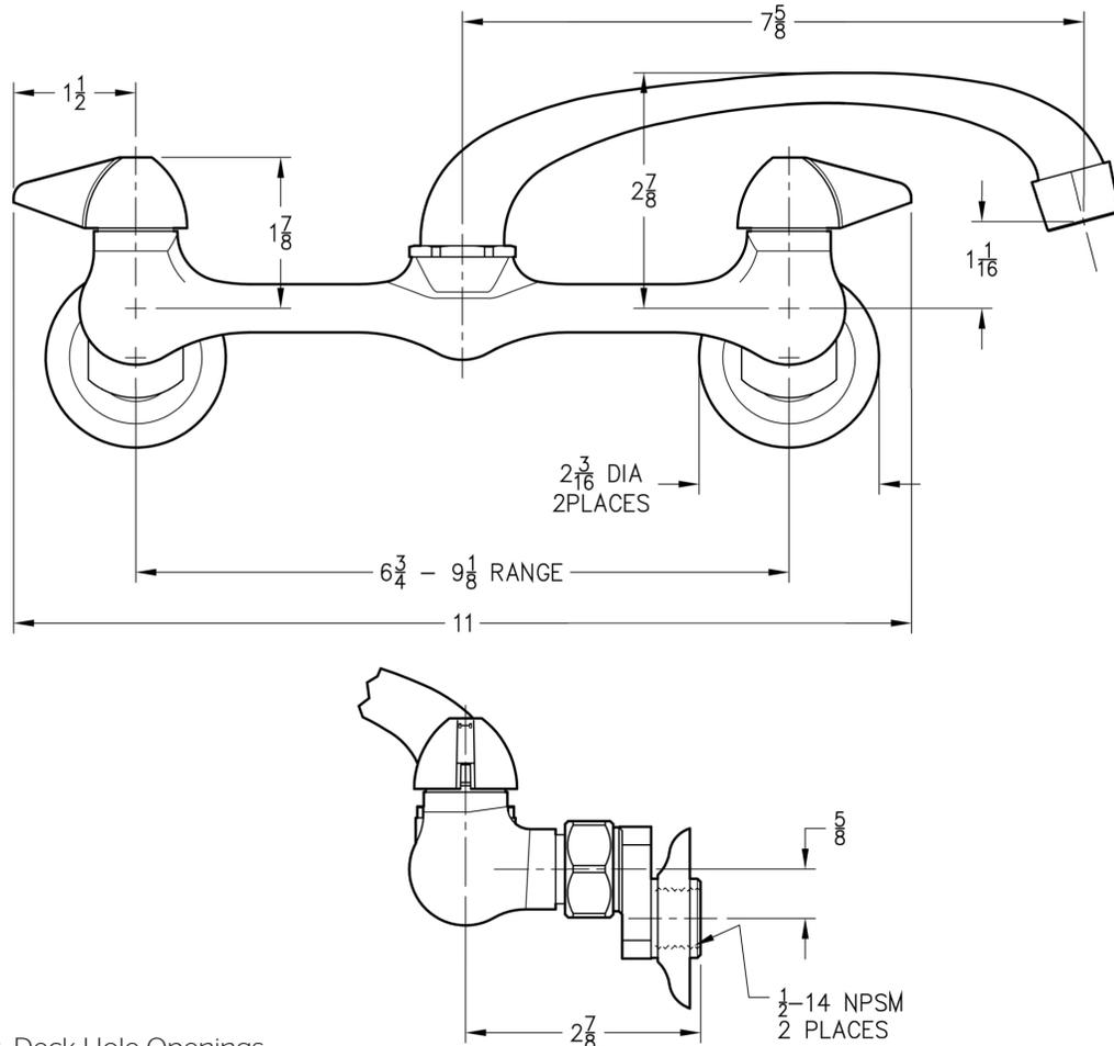
Ø1-3/8 Min to Ø1-1/2 Max. Deck Hole Openings
