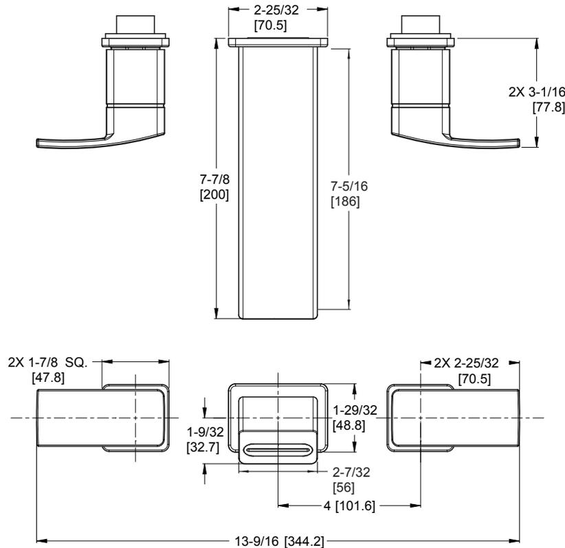
Ø1 Min to Ø1-1/2 Max. Deck Hole Openings
