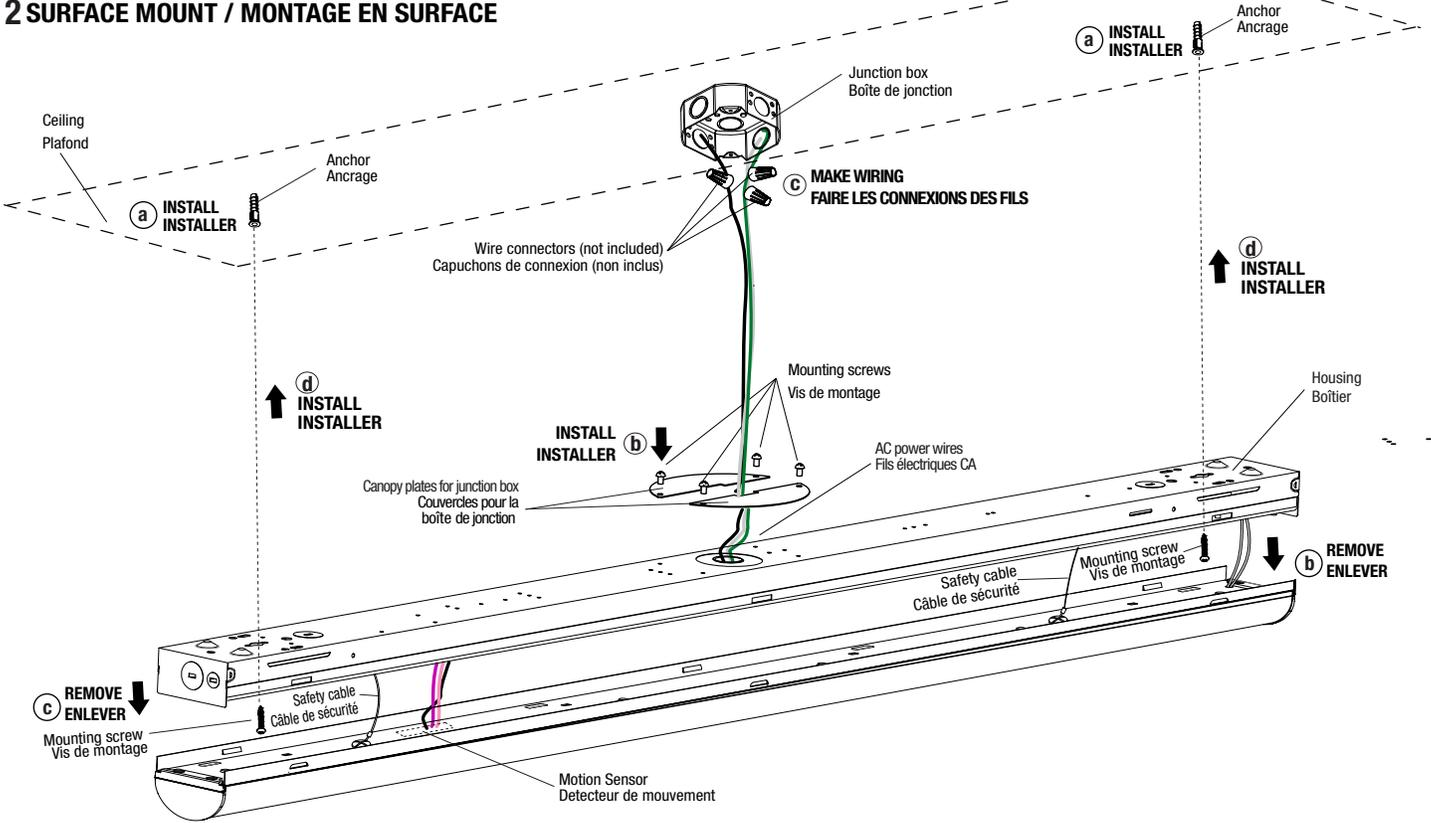
**SURFACE MOUNT INSTALLATION DIMENSIONS FOR 3 FT AND 4 FT LUMINAIRES
