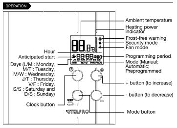
The multiple programming thermostat has three main operating modes: Manual (**MRN**), Automatic (**AUTO**) and Preprogrammed (**PRE-PROG**). The active mode is displayed at the bottom of the screen. The transition from one mode to another is done by pressing down the **MODE** button, out of any adjustment mode.
