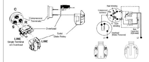
Terminal No.1: Attach one side of run capacitor here if present, if not leave terminal open. Terminal No.2: Attach one side of the 120 VAC line here
