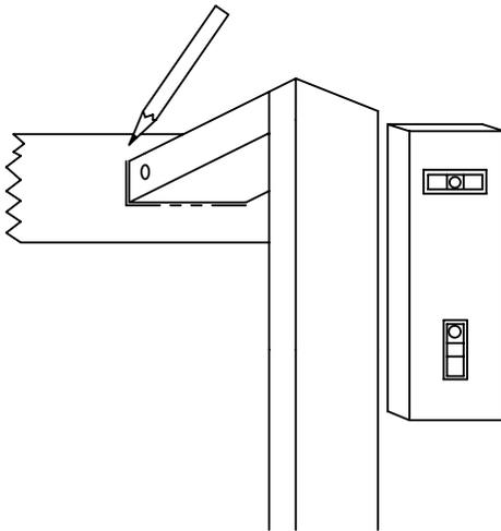
7. POSITION THE RAIL UPRIGHT AND USE A LEVEL TO ENSURE THAT IT IS VERTICAL. TIGHTEN THE SET SCREW TO SECURE THE RAIL TO THE WATERWAY ELBOW.
