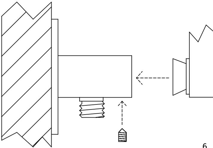
6. SLIDE THE ROUND ANCHOR MOUNTED ON THE RAIL INTO THE HOLE IN THE FRONT OF THE WATERWAY ELBOW. INSERT THE SET SCREW.
