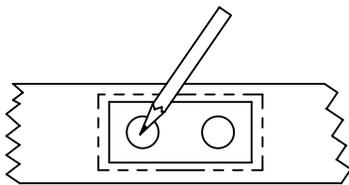
10. PLACE THE RECTANGULAR BRASS INSERT AGAINST THE WALL, IN THE CENTER OF THE OUTLINE FROM THE PREVIOUS STEP.
