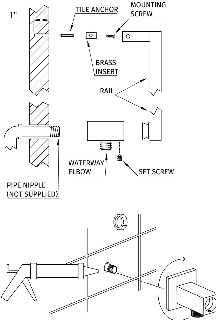
1. USE THE INCLUDED ALLEN KEY TO REMOVE THE WATERWAY ELBOW FROM THE BOTTOM OF THE RAIL AND THE BRASS INSERT FROM THE TOP.
