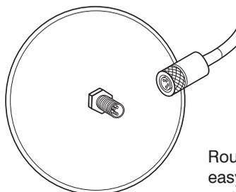
Route the data cable (included with easy start) through the finished wall to the back side of the control. The other end of the cable runs to the Y-connector. See possible configurations in step 5.
