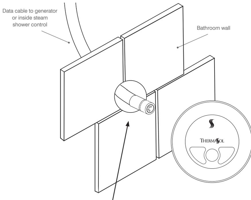
Make a 1/2" diameter hole in the desired location.
