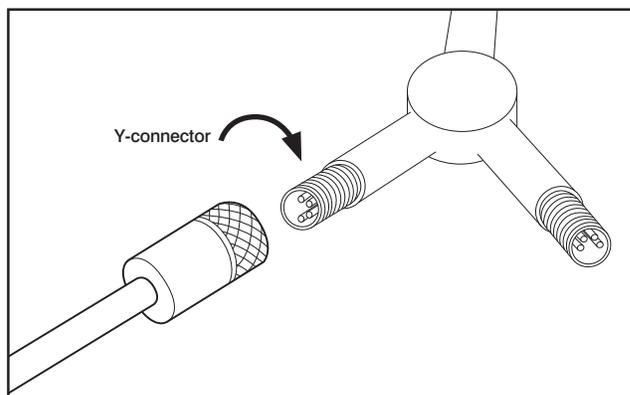
Connect the data cable to Y-connector. (The other ends of the cables run to the back of the control in the shower or the PDM if present.)
