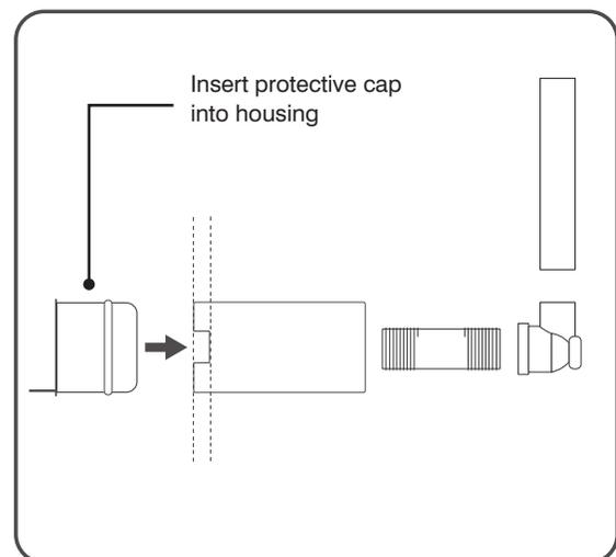
**D** Once the shower wall is complete and the housing is sealed to the wall, remove the protective cap and insert the steamhead into housing. Use the supplied silicone to adhere the steamhead to the wall sealing out any water from getting behind the head.
