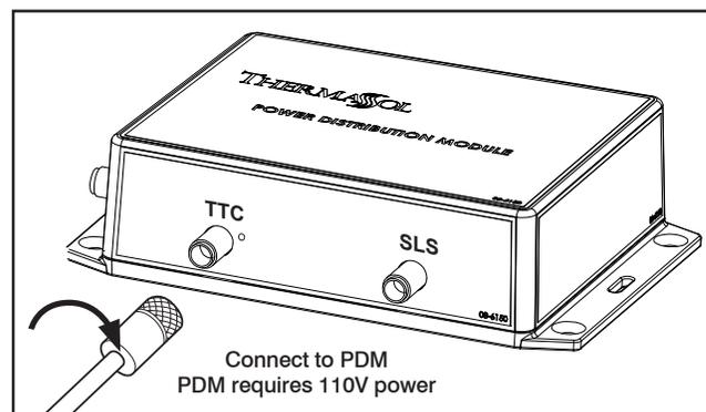
Connect the data cable to Power Distribution Module (PDM). (The other end of the cable runs to the back of the control in the shower location.)
