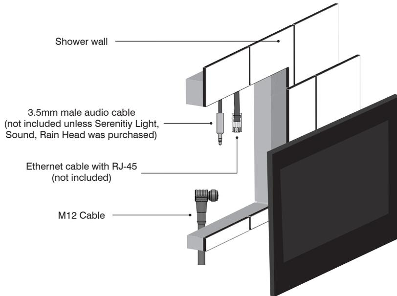
Route the M12 cable through the finished wall to the back side of the control. (The other end of the cable runs to the PDM location.) **NOTE:** It is recommended to run the cable through electrical conduit. **DO NOT STAPLE** the cable!
