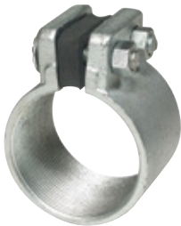
ABB's split coupling is a simple method to join threaded conduits in retrofits or in snug areas. Available in ½" to 6".
