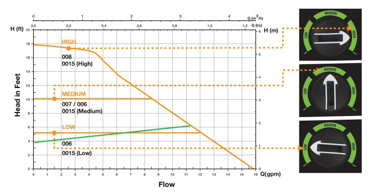
The 0015e3 circulator provides three constant pressure settings to match system requirements. Selection options are **LOW** (5 feet), **MEDIUM** (10 feet), or **HIGH** (18 feet). See chart above for the equivalent 00° model at each setting.
