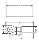
These heat shrinkable products provide a tough, environmentally sealed wire termination. These terminals and splices insulate and protect the electrical connections from wire pull-outs, abrasions and mechanical abuse. They also resist water, salt and other contaminants.
