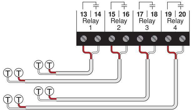
**Wiring the Boiler Pumps**
