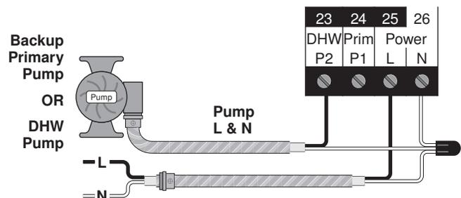
**Wiring the Modulating Boiler Outputs**
