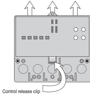
Press the control release clip on the base inside the wiring chamber and slide the control upwards.
