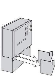
Remove the safety dividers from the wiring chamber by pulling them straight out of their grooves.
