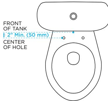
2. Minimum of 2 inches\*\* (50 mm) from front face of tank to the center of mounting holes.
