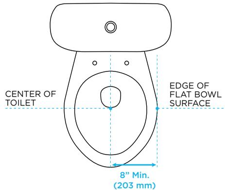
4. Minimum of 8 inches (203 mm) of open space from center of toilet to edge of flat bowl surface.
