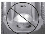
OVAL NECK OF BOLT NOT SEATED PROPERLY
