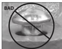
OVAL NECK OF BOLT NOT SEATED PROPERLY
