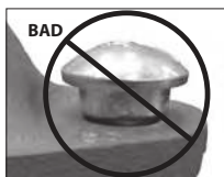
OVAL NECK OF BOLT NOT SEATED PROPERLY
