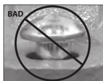
OVAL NECK OF BOLT NOT SEATED PROPERLY
