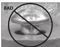
OVAL NECK OF BOLT NOT SEATED PROPERLY
