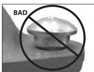
OVAL NECK OF BOLT NOT SEATED PROPERLY
