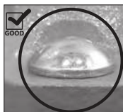
OVAL NECK OF BOLT SEATED PROPERLY
