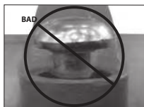
OVAL NECK OF BOLT NOT SEATED PROPERLY
