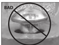
OVAL NECK OF BOLT NOT SEATED PROPERLY
