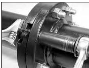
4-Bolt Tightening Pattern
