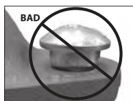
OVAL NECK OF BOLT NOT SEATED PROPERLY
