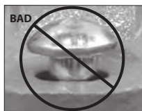
OVAL NECK OF BOLT NOT SEATED PROPERLY
