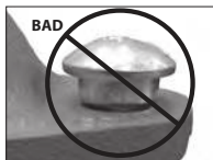
OVAL NECK OF BOLT NOT SEATED PROPERLY
