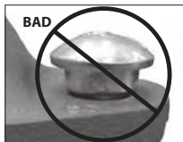
OVAL NECK OF BOLT NOT SEATED PROPERLY
