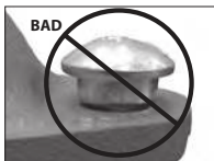
OVAL NECK OF BOLT NOT SEATED PROPERLY
