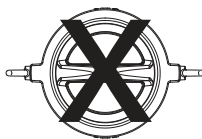
Incorrect Orientation for Horizontal Installation
