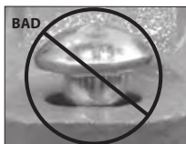
OVAL NECK OF BOLT NOT SEATED PROPERLY
