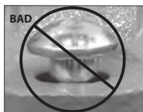
OVAL NECK OF BOLT NOT SEATED PROPERLY
