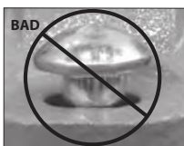
OVAL NECK OF BOLT NOT SEATED PROPERLY
