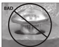
OVAL NECK OF BOLT NOT SEATED PROPERLY
