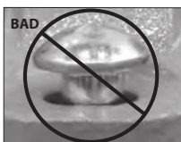
OVAL NECK OF BOLT NOT SEATED PROPERLY
