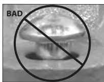
OVAL NECK OF BOLT NOT SEATED PROPERLY
