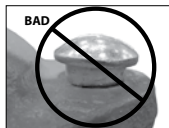
OVAL NECK OF BOLT NOT SEATED PROPERLY
