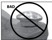
OVAL NECK OF BOLT NOT SEATED PROPERLY
