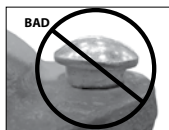
OVAL NECK OF BOLT NOT SEATED PROPERLY
