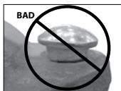
OVAL NECK OF BOLT NOT SEATED PROPERLY
