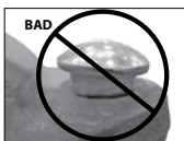
OVAL NECK OF BOLT NOT SEATED PROPERLY
