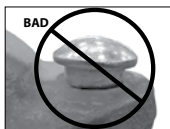
OVAL NECK OF BOLT NOT SEATED PROPERLY
