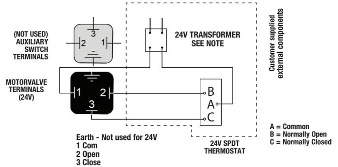
NOTE: 1/4" - 2" EMVII-6400SS-24-40 will operate with a 40 VA transformer. Thermostat must be capable of handling amp rating at stall.
