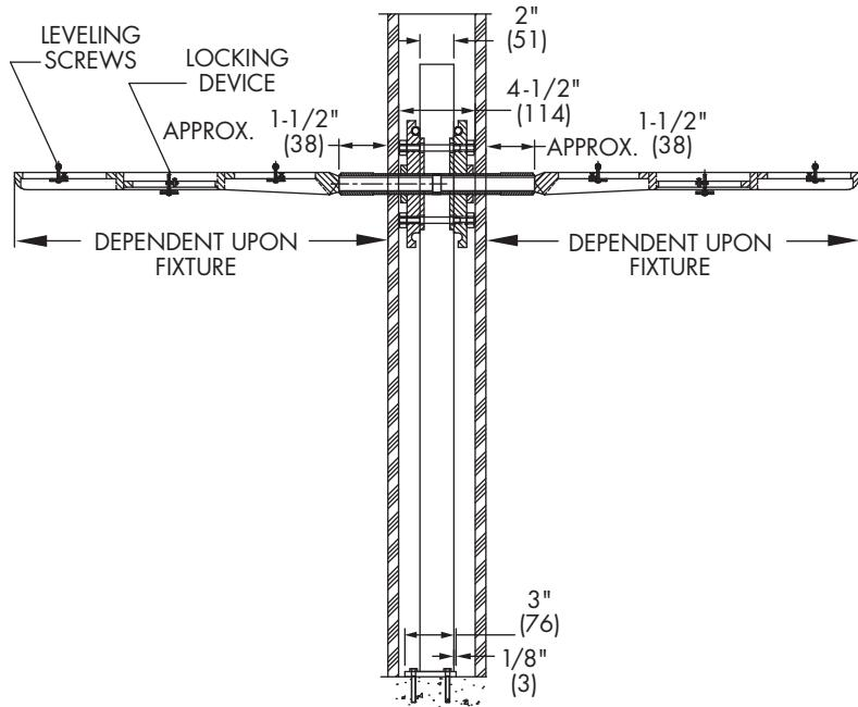
**Note:** Anchor legs to concrete floor with minimum 1/2" anchor bolts (by others).
