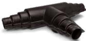
**Protective Tee Casing for R-flex** — For waterproof sealing and insulating of tee connections. Includes 2 HDPE halves, insulation, sealer kit, and bolts. Must add shrink caps to seal ends of R-flex.
