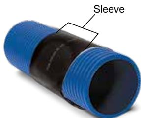
**R-flex Jacket Repair Sleeve** — To repair accidental damage to R-flex outer cover. Slide the sleeve over damaged area and heat with heat gun.
