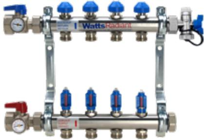
**Stainless Steel manifolds** are made of heavy-walled stainless steel. Matching fittings and accessories are made of solid brass and are heavily plated with nickel to match the appearance of the manifold trunk. Standard features included flow balancing valves, circuit isolation valves, and flow meters. Manifolds are sold in pre-mounted pairs in 1" and 1 1/2" Hi Flow sizes.
