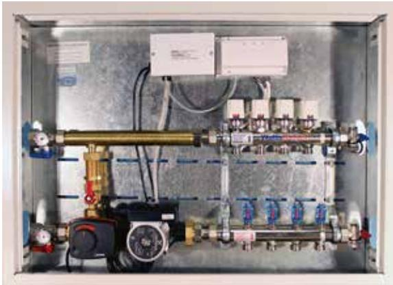
The ThermalPro Isotherm Mixing Module is a compact, pre-piped, pre-wired pump and mixing valve control connected directly to a Watts 1" Standard or 1-1/2 Hi-Flow Stainless Steel manifold and installed in a white powder coated steel cabinet with cover door.
