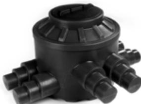
**Protective Inspection Chamber for R-flex** — Allows access to connections and/or valves. Includes HDPE chamber with 6 connection points, inspection lid, sealer kit and screws. Must add shrink caps to seal ends of R-flex, and jacket repair sleeves for sealing the R-flex to the chamber.
