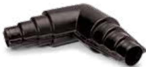
**Protective Elbow Casing for R-flex** — For waterproof sealing and insulating of elbow connections. Includes 2 HDPE halves, insulation, sealer kit, and bolts. Must add shrink caps to seal ends of R-flex.
