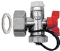
This assembly allows for the purging of zones at the manifold location. It includes 3/8" manual air vent and a 1/2" ball valve with GHT for the supply and return. Nickel plated brass.
