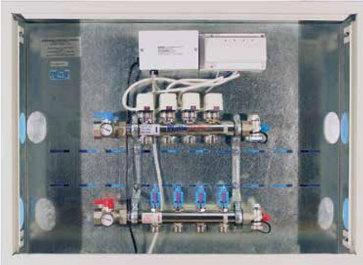
The ThermalPro Non-Mixing Manifold Station consists of either a Watts 1" Standard or 1 1/2" HiFlow Stainless Steel manifold installed in a beautiful white powder coated steel cabinet with cover door. Manifold Stations are available in 2 to 12 loop manifold configurations. The Manifold Station can be provided with manifold loop actuating motors and a Watts Zone Control Module installed in the cabinet to simplify system zone wiring.
