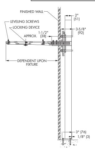
Note: Anchor legs to concrete floor with minimum 1/2" anchor bolts (by others).
