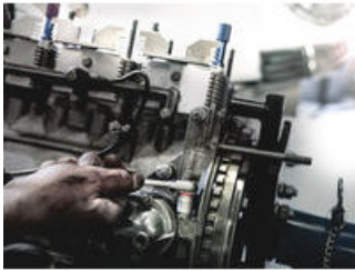
Nutsetter for hexagon head screws
