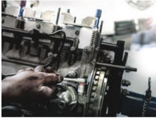
Nutsetter for hexagon head screws
