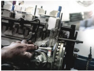
Nutsetter for hexagon head screws
